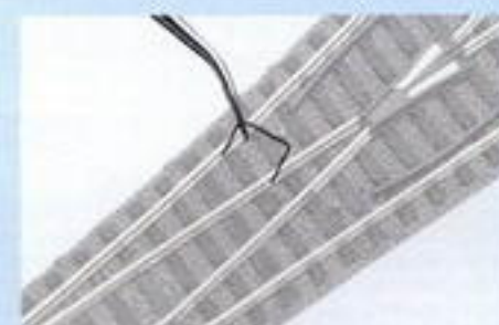
By removing the wire bridge-clips FLEISCHMANN points become "thinking" points with stop function.
